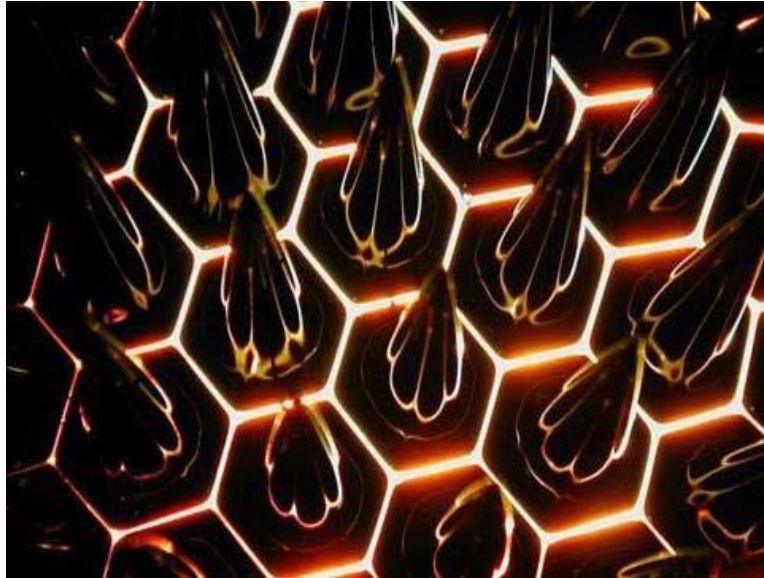
Figure 1-4: The hexagonal peaking patterns produced by ferrofluids that are exposed to perpendicular magnetic fields, 33 mT in this case [11].
